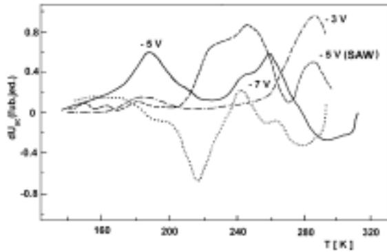
Fig. 2. A-DLTS spectra of GaAs/AlGaAs heterostructures obtained from ARS and TAS transients as function of bias gate voltage for relaxation time  $\tau = 43.6$  ms
