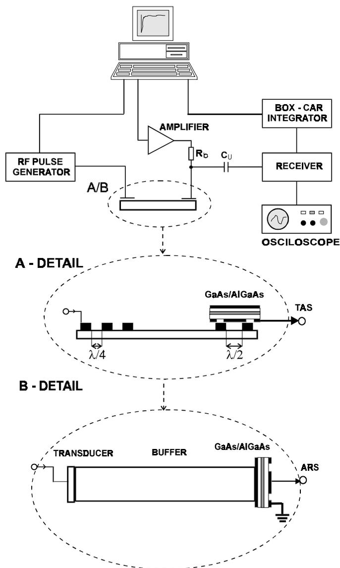
Fig. 1. Block diagram of the experimental arrangement for A-DLTS measurements. The detailed configuration is illustrated in A-detail (TAS measurement) and B-detail (RAS measurement).
